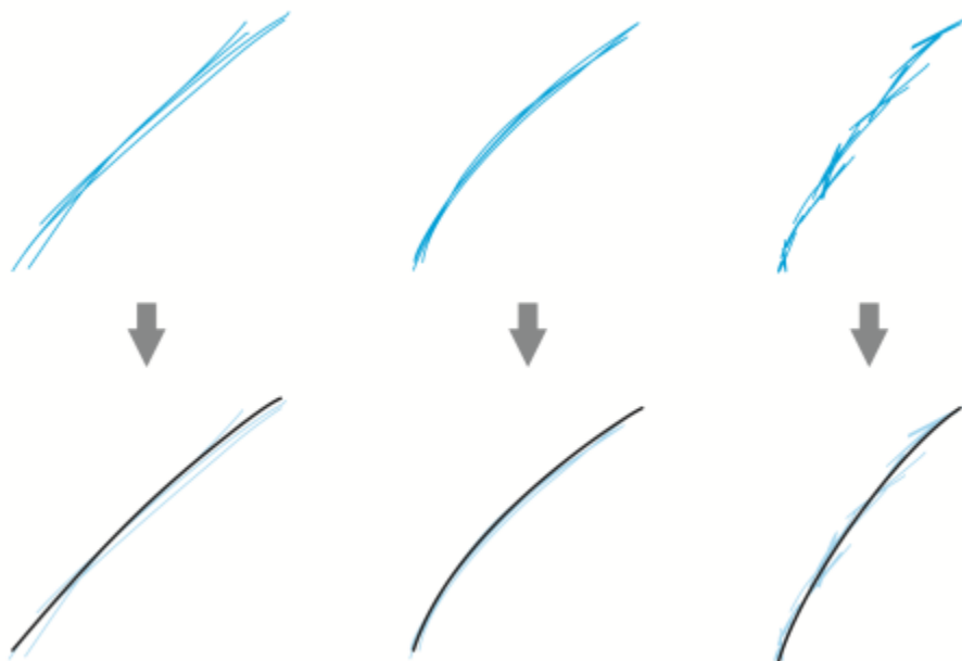
Strokes before (top) and after (bottom) stroke adjustment: discrete overlapping strokes (left), folded strokes (middle), chicken scratch (right)
