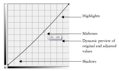
The tone curve shows the balance between the shadows, midtones, and highlights of an image. The original (x) and adjusted (y) pixel values are displayed side by side when you drag the tone curve. This example shows a small adjustment to the tonal range, in which pixel values of 152 are replaced with pixel values of 141.
