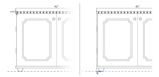
5 To change the dimension text for the height, double-click the dimension text by using the **Text** tool , and type **19**".
