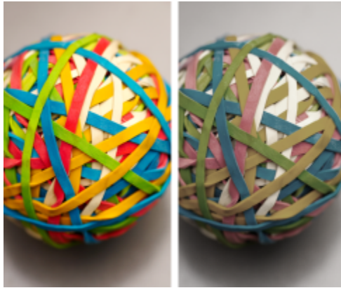
Left: The SWOP 2006_Coated3v2.icc color profile is assigned to the active document. Right: When the Japan Color 2002 Newspaper color profile is assigned to the document, the colors appear much less saturated.
