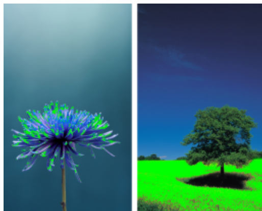
The number of out-of-gamut colors (indicated by the green overlay) may influence your choice of a rendering intent. Left: The Relative colorimetric rendering intent is suitable for this photo, which contains only a few out-of-gamut colors. Right: The Perceptual rendering intent is a good choice for this photo, which contains many out-of-gamut colors.
