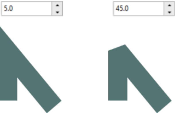
Lines meet at the same sharp angle. Left: The angle exceeds the miter limit, creating a pointed corner. Right: The angle is below the miter limit, creating a beveled corner.
